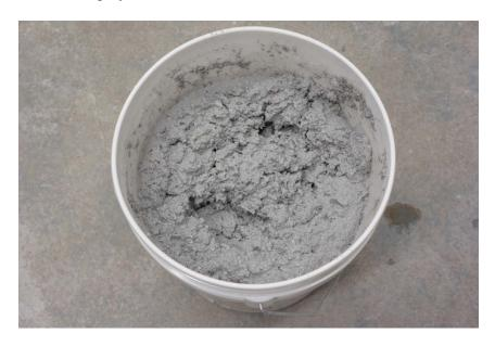
When properly mixed, Monokote Patch Compound has a potlife between 2 to 4 hours. Monokote Patching Compound should not be retempered if the material has started to stiffen or set.
