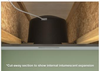
The FF109-350 is **the larger version** of the FF109-300. Both covers are made out of the same intumescent material and exhibit excellent **thermal and acoustical** insulating properties. The FF109-350 has an inside height of 10 3/8" and a diameter of 15" to fit the most common recessed light housings.
