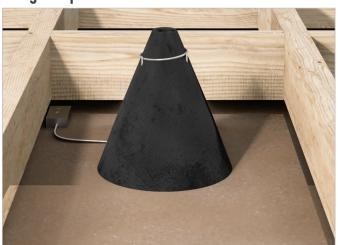
The FF109-250 is a cone-shaped intumescent enclosure which has been specifically designed to help protect openings for **6**<sup>7</sup> **low profile LED downlight fixtures**. The ultra-flexible nature of the material allows the cover to get rolled up for easy retrofit, remodel or new construction installation from below the ceiling and provide a 60 minute flame, smoke and heat barrier.
