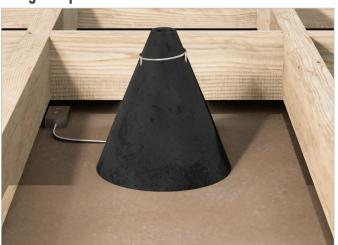
The FF109-200 is a cone-shaped intumescent enclosure which has been designed to help protect openings for **4**<sup>*n*</sup> **low profile LED downlight fixtures**. The high expansion and insulating properties of the material ensure that both, flame spread and heat transmission, are stopped for 60 minutes. The **flexible material** allows the cover to get rolled up for easy retrofit or new construction installation.
