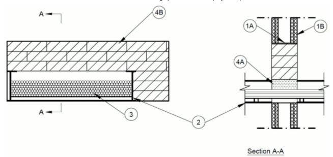
1. Wall Assembly — The 1 or 2 hr fire rated gypsum board/steel stud wall assembly shall be constructed of the materials and in the manner described in the individual U400, V400 or W400 Series Wall and Partition Designs in the UL Fire Resistance Directory and shall incorporate the following construction features:
