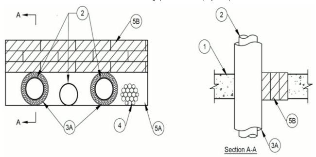
1. **Floor or Wall Assembly** — Min 4-1/2 in. (114 mm) thick reinforced lightweight or normal weight (100-150 pcf or 1600-2400 kg/m<sup>3</sup>) concrete. Wall may also be constructed of any UL Classified **Concrete Blocks\*.** Max area of opening is 384 in.<sup>2</sup> (2477 cm<sup>2</sup>) with a max dimension of 32 in. (813 mm).
