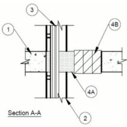
1. **Floor or Wall Assembly** — Min 4-1/2 in. (114 mm) thick reinforced lightweight or normal weight (100-150 pcf or 1600-2400 kg/m<sup>3</sup>) concrete. Wall may also be constructed of any UL Classified **Concrete Blocks\*.** Max area of opening is 384 in.<sup>2</sup> (2477 cm<sup>2</sup>) with a max dimension of 32 in. (813 mm).
