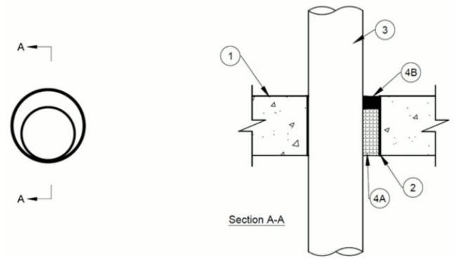
1. Floor or Wall Assembly — Min 4-1/2 in. (114 mm) thick reinforced lightweight or normal weight (100-150 pcf or 1600-2400 kg/m<sup>3</sup>) concrete. Wall may also be constructed of any UL Classified Concrete Blocks\*. Diameter of opening is maximum 5 in (127 mm).
