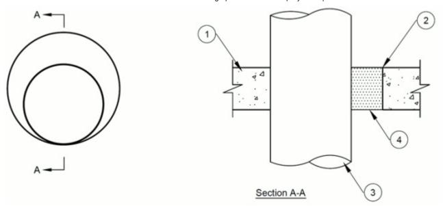
1. Floor or Wall Assembly — Min 4-1/2 in. (114 mm) thick reinforced lightweight or normal weight (100 - 150 pcf or 1600-2400 kg/m<sup>3</sup>) concrete. Wall may also be constructed of any UL Classified **Concrete Blocks\***. Max diam of opening is 12 in. (305 mm).
