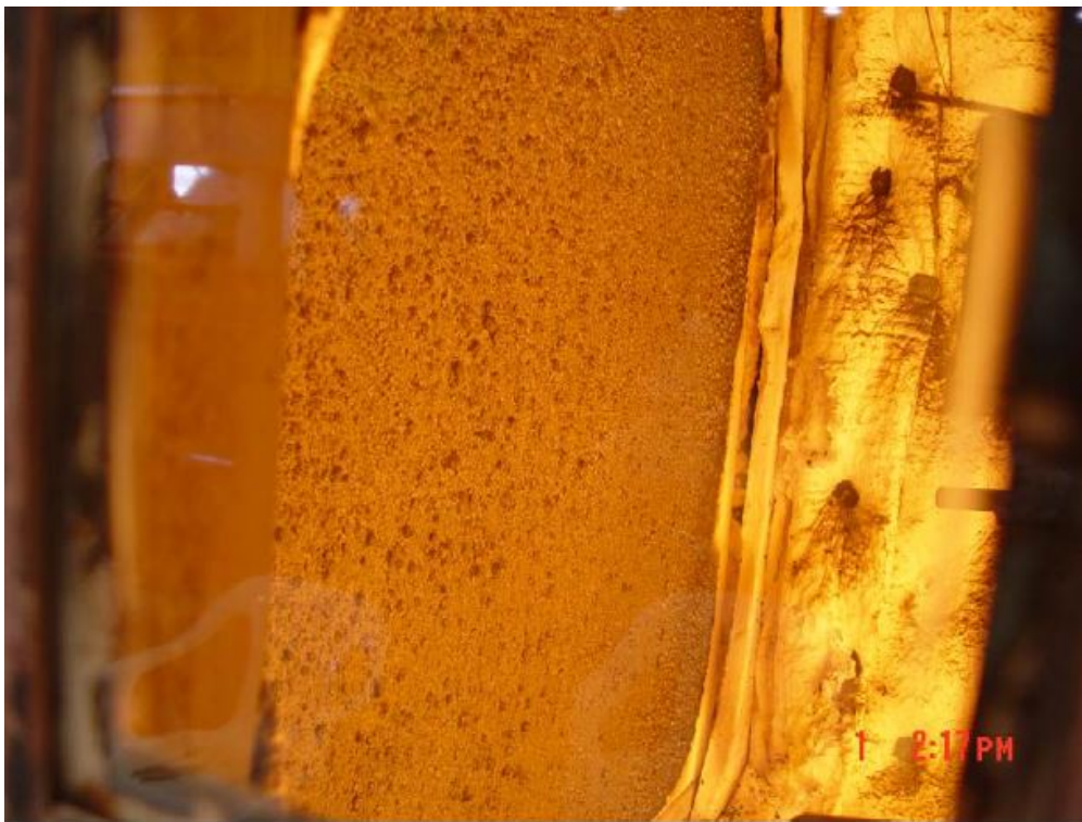
Photograph 3: Sample exposed face beginning to intumesce
