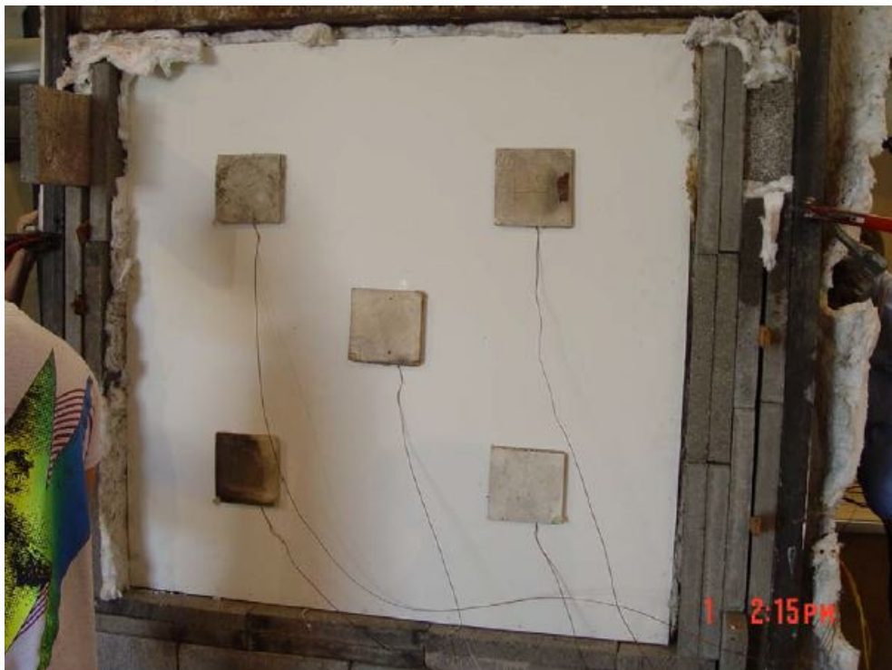
Photograph 2: Sample unexposed face pre-test, showing thermocouples
