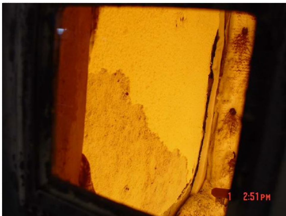
Photograph 4: Large pieces of intumescent falling from exposed face
