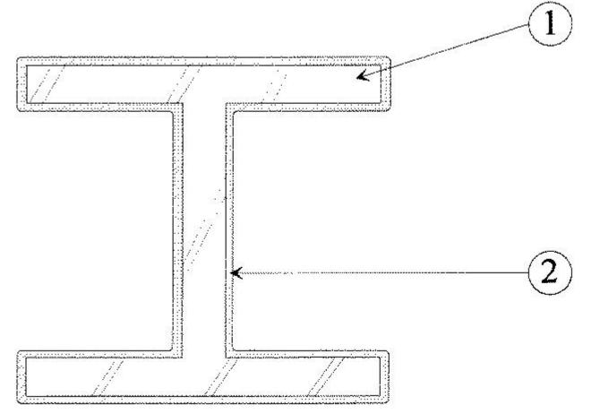
1. **Steel Column** — Min size shown in table below. The column surfaces shall be free of dirt, loose scale and oil. Steel surfaces to be primed with a red oxide primer as required per manufacturer's application instructions.
