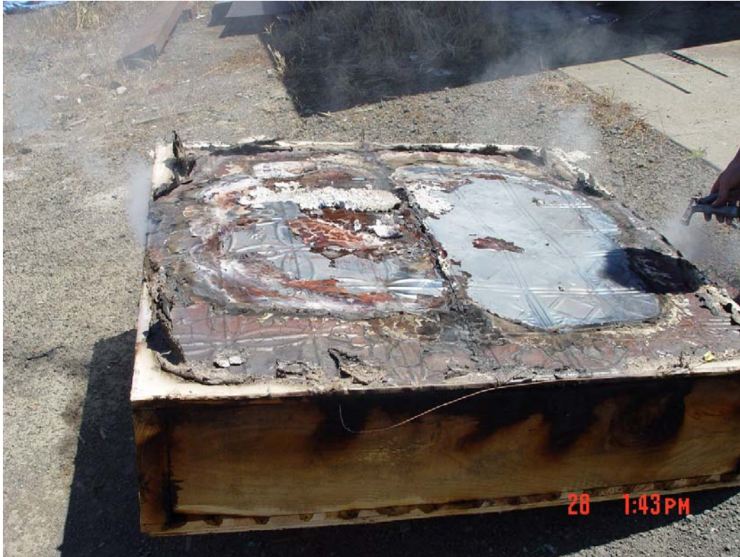
Photograph 9: Exposed face of the sample post-test
