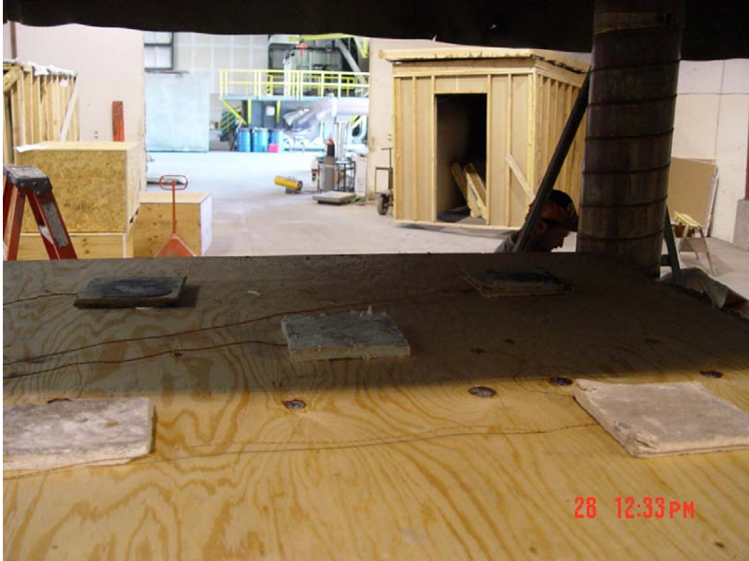
Photograph 3: Unexposed sample face pre-test showing thermocouple placement
