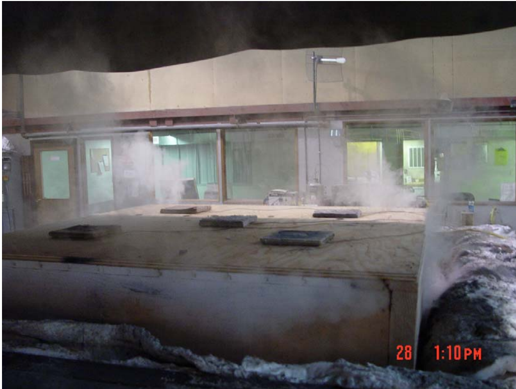
Photograph 7: Unexposed face of the sample during test
