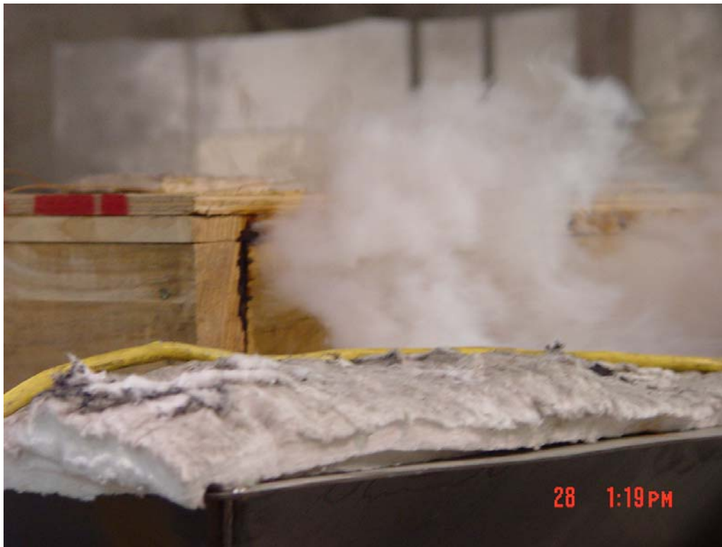
Photograph 8: Smoke shooting from a gap in the frame of the sample
